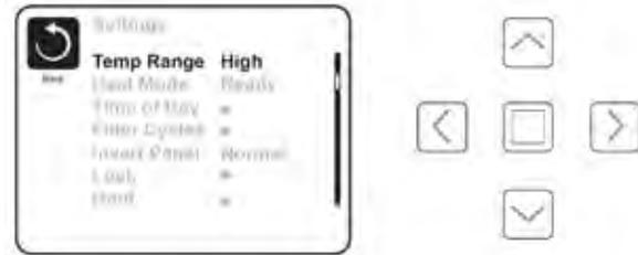
When in “Ready” mode, the pump that circulates water through the heater will turn on every 1/2 hour to measure water temperature, heat if needed, and refresh the temperature display. When in Ready mode your spa will continually maintain its set temperature. REST mode is recommended for most economic performance.
