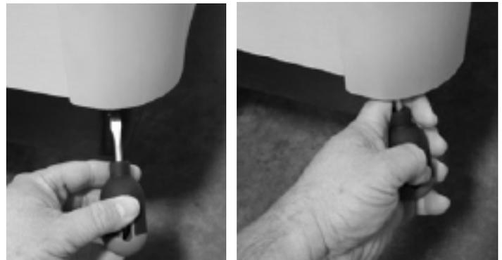
remove the door, start by placing a longer flathead screwdriver or short pry bar into the center of the snap feature and use it as a lever to pop the door out of the first snap. Grab the base of the door and carefully begin pulling it out such that the rest of the snaps come free one by one across the length of the door. The door can then be dropped out of the groove on top and removed from the spa.
