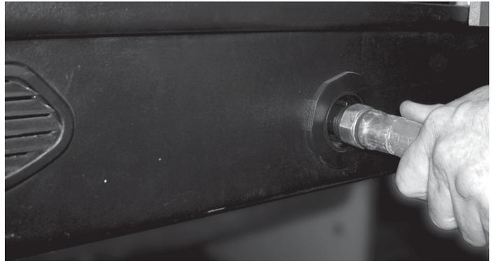
**Step 6:** Once the spa is fully drained, pull the drain spout out all the way, remove hose, replace the drain cap and push drain in all the way.
