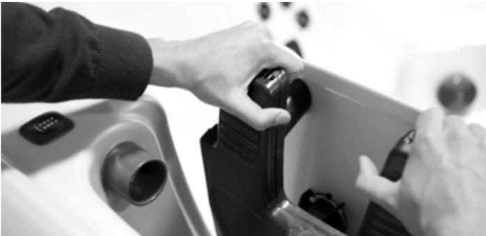
**Step 5:** Lower the manifold of the new JetPak carefully as to align the lower valve assembly and gasket into the bulkhead fitting. Apply pressure downward as you pull the JetPak manifold toward you to until the manifold is secured in the wall clip assembly .
