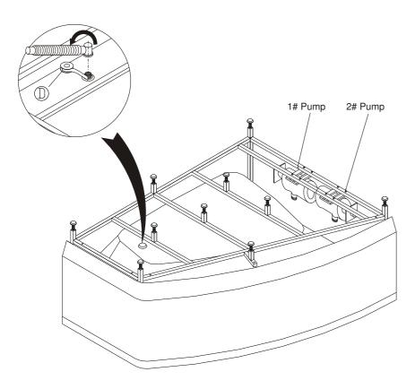
2. As the below picture: Turn back the bathtub. Then Install the water-inlet waterfall and handheld shower on and connect to the water hose. Move the bathtub to the wall corner. Put the downcomer into the drain hole. And use sealant around the hole. Adjust the anchor screw to make the bathtub horizontal.
